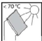
When the sun shines, the collectors can become very hot. The solar fluid in the circuit can heat up to more than 100 °C. Only flush and fill the solar circuit when the collector temperatures are below 70 °C.
