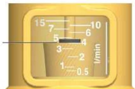
1. Set the desired maximum flow rate at the controller
