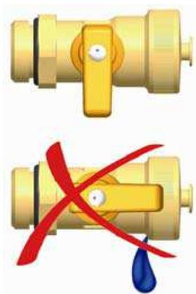
11. Remove the hoses of the flush and fill station and screw the sealing caps onto the fill and drain valves. The sealing caps only serve to protect the valves against dirt. They are not designed to take up high system pressures. The ball valves must be closed to guarantee tightness
